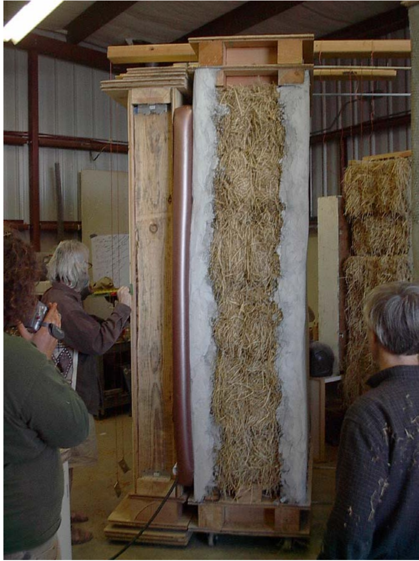
Rig docked to cement-plaster (stucco) straw-bale wall
