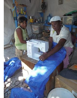
Tarps into gravel bags
