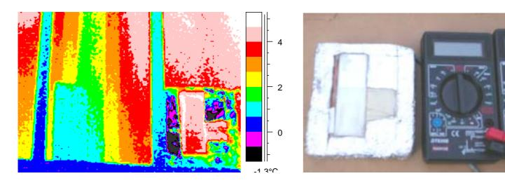
Black temperatures. Unheated reference piece of glass at left, the heated one at right, standing on a window grate.
