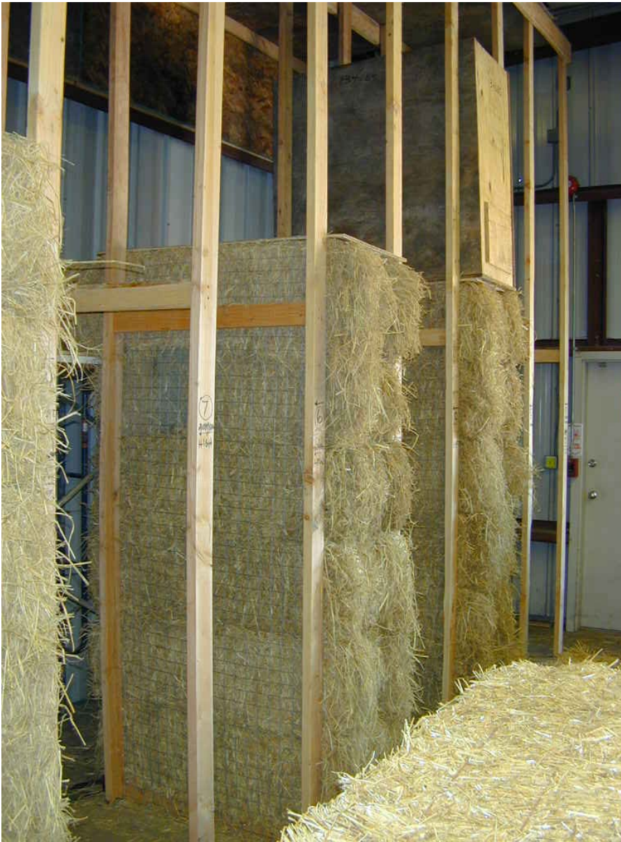
Photo #1: Creep test stack assembly, showing Stacks 8, 5, and 3.
