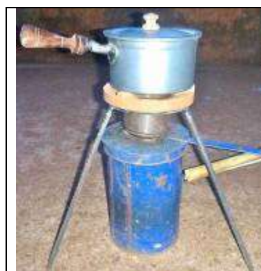
A Champion reactor made in Malawi with movable tripod-stand for the pot (Photo: Christa Roth)
