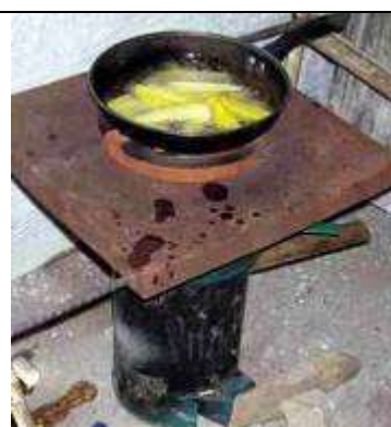
A Champion reactor made in Mozambique with a fixed stand for the pot
