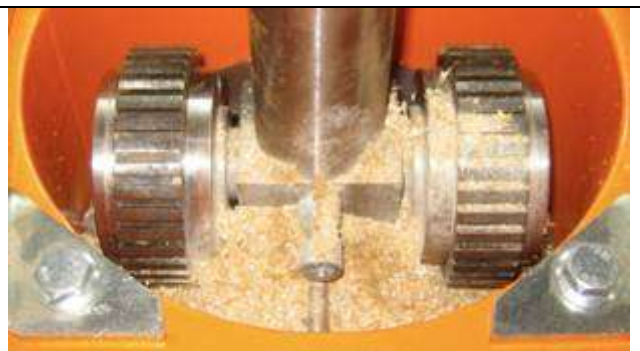
Rollers pushing sawdust through the holes of a small 210 mm diameter flat-die disk below. Photos displaying an Ecoworxx Pelletiser
