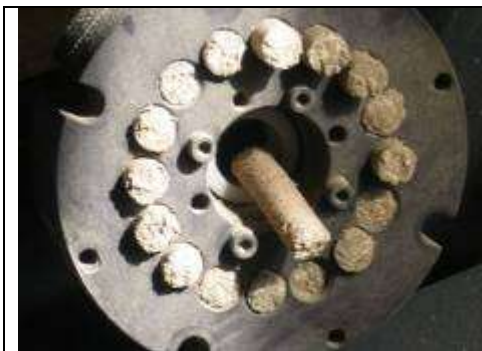
'Maxi-pellets' pressed through 20-mm-holes of a flat-die at a rate of 50-80 kg/h, depending on material
