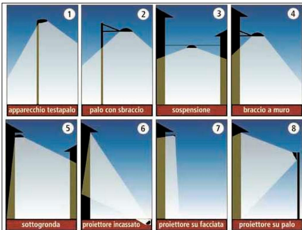
Fig.3 -- Lighting installations corresponding to the r.l. 17/00 requirements. The lighting devices as from points 6 and 8 are admitted by the r.l. 17/00 art.6 paragraph 10 exclusively for structures of particular and proved historical importance only if it is not possible light up them from upward.
