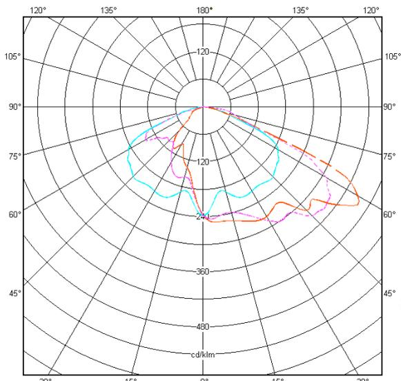
Fotometric curve for Asymmetrical optics
