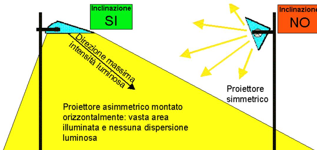
[Symmetric and asymmetric devices if placed horizontally and with flat protective glass are equally conform to the R.L. 17/00 ]
