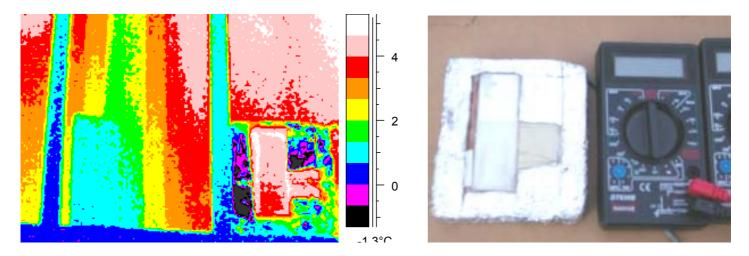
Black temperatures. Unheated reference piece of glass at left, the heated one at right, standing on a window grate.
