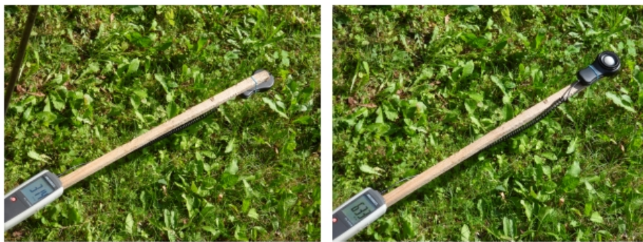
Figure 4: Measuring solar albedo of grass using PV solarmeter. The sensor placed 30 cm above ground detects radiation reflected by grass surface (left) and incident solar radiation (right). The same procedure is applied to measure visual albedo using luxmeter.
