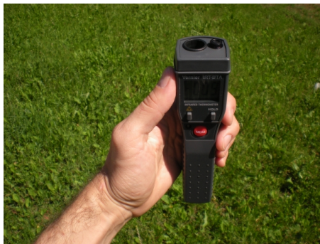
Figure 1: Measuring LWIR temperature of the zenith sky using infrared thermometer.
