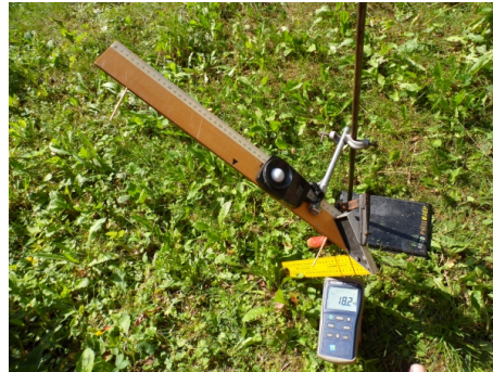
Figure 2: Verifying lambertian (cosine) sensitivity of a luxmeter sensor.
