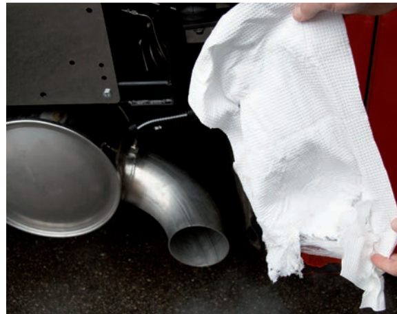
The combination of closed particulate filters and city-SCR systems effectively remove both particles and nitrogen oxides from the exhaust.
