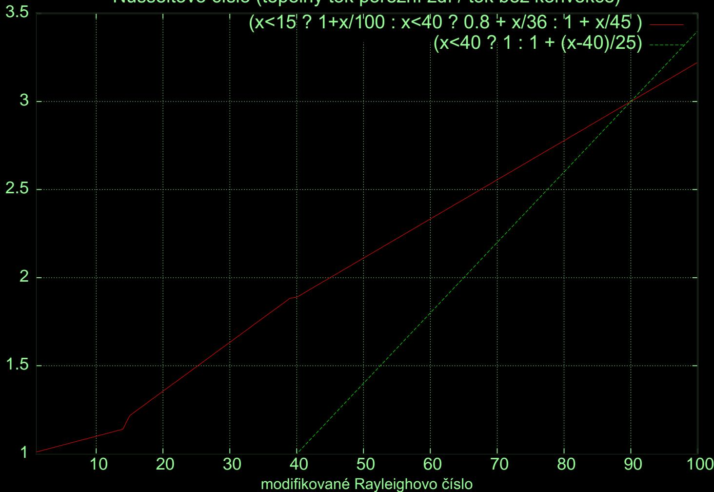
$$Ra_m = 0,7 \frac{H}{1\text{ dm}} \frac{T}{10\text{ K}} \frac{K}{0,01\text{ mm}^2}$$
