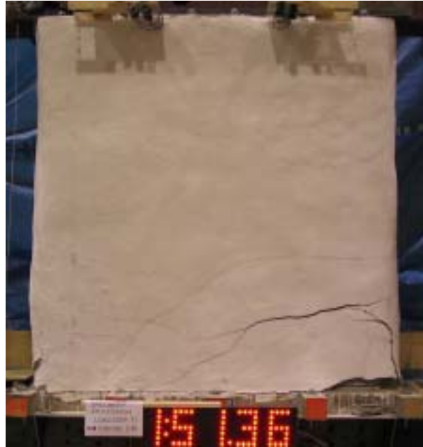
Figure 6.11 – Wall F flexural cracks (2.5% drift level)
