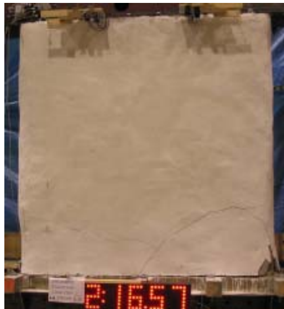
Figure 6.8 – Flexural cracks in Wall E (2.5% drift level)
