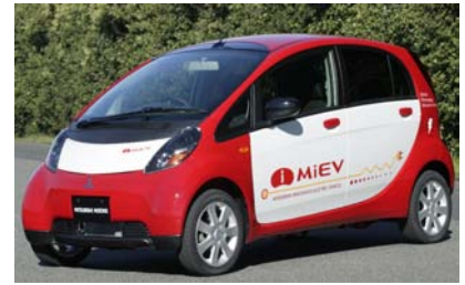
Figure 20.38. The i MiEV from Mitsubishi Motors Corporation. It has a 47 kW motor, weighs 1080 kg, and has a top speed of 130 km/h.
