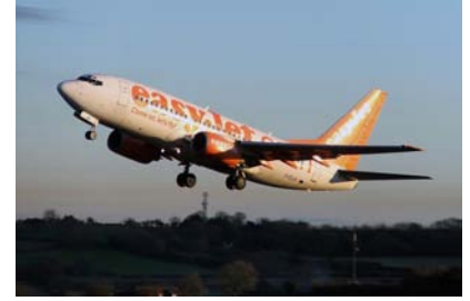
Figure C.11. Boeing 737-700: 30 kWh per 100 passenger-km. Photograph © Tom Collins.
