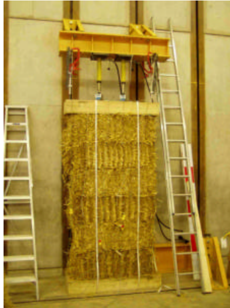
Figure 3 Static load test
