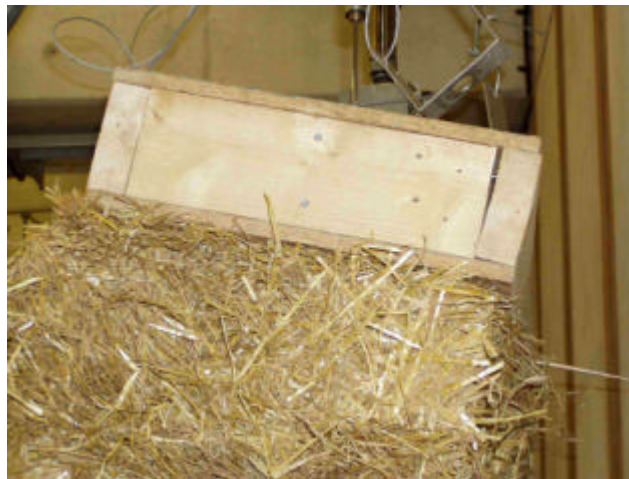
Figure 7 Rotation of wall plate
