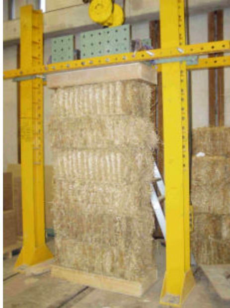
Figure 2 Settlement test set-up
