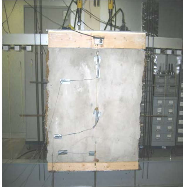
Figure 4.6 – Improved test setup with potentiometers attached to box beam
