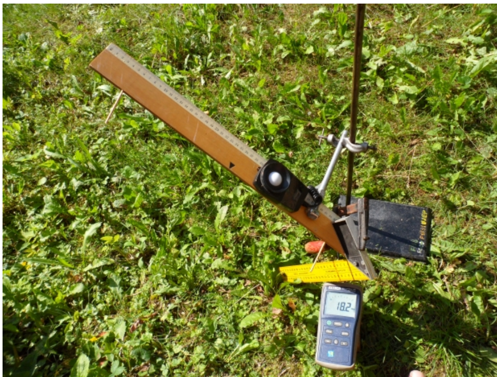
Figure 5.6: Verifying Lambertian (cosine) sensitivity of a luxmeter sensor. Instead of the shadow of a rod, the shadows of two sticks inserted into the ruler are used, as the centres of their shadows are unequivocal.
