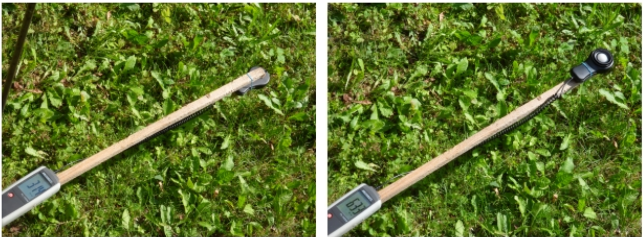
Figure 5.8: Measurement of solar albedo of forbs and grasses using a sun-meter in non-variable conditions (cloudless sky). The sensor is kept 3 dm above the ground. The image on the left shows the radiation returned upwards being recorded; the one on the right one depicts the recording of incident solar radiation. The same procedure is used for measuring visual albedo with a luxmeter. Attaching the sensor to a 1 m lath is better than holding the sensor in your hand, as you, the observer will be farther from sensor, which will limit the the influence of your shadow. Of course, you should stand so that your shadow goes away from the sensor.
