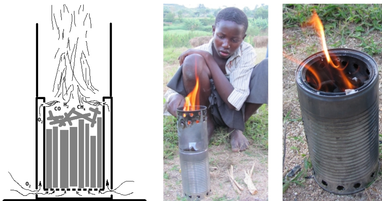
Figure 6.2: Scheme of wood gas stove TLUD (left), real TLUD stove from three cans (middle) and detail of flames where wood gas mixes with preheated air (right).
