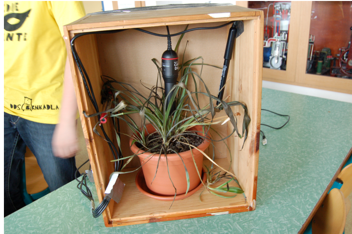
Figure 7.4: An assembly of a plant and sensors in a box after the experiment. The plant is damaged by extreme conditions due to sunshine/temperature.
