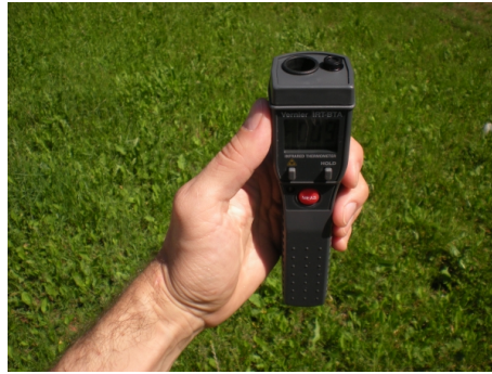
Figure 5.5: Measuring the LWIR temperature of the sky near zenith using an IR thermometer
