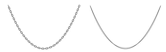
Figure 13: Left: The catenary, or shape of a hanging chain, which Galileo erroneously believed to be a parabola. Right: The catenary (dotted) compared to a parabola (solid) of equal arc length between the same endpoints.
