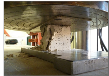
Concrete samples being made . . . and then crushed to test strength.
