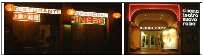
Fig.22 - A few types of signboards exempted by the law and for which the law requires, but only in the protected zones, only the switching off after 23.00 hours or at the time of closing of the exercise. It is possible to see: boxed letters with their own lighting (the cinema inscription), uncovered neons (entry decoration at the cinema and inscription in Chinese), or panels with internal lighting (the inscriptions restaurant and the playbill of the cinema).
