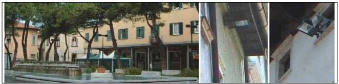
Fig.11 – Left: Dalmine City Hall Square. Lighting corresponding to the R.L. 17/00 requirements and light sources placed so as not to interfere with the trees canopy. Right: Two examples of lighting of old cities centres with devices under eave (in the image to far right a horizontal device put beside to an inclined one which instead disperses light upwards).
