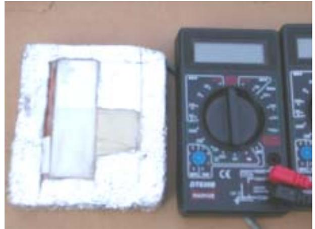
*Black temperatures. Unheated reference piece of glass at left, the heated one at right, standing on a window grate.*
