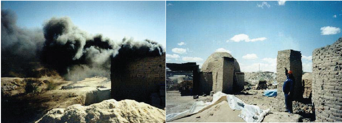
Figure A.5.4. Left: Firing of a conventional kiln in Ciudad Juarez, Chihuahua, Mexico (Photograph courtesy of Robert Marquez). Right: Firing of a Marquez kiln in Ciudad Juarez, Chihuahua, Mexico. (Photograph courtesy of Alba Corral Avitia).
