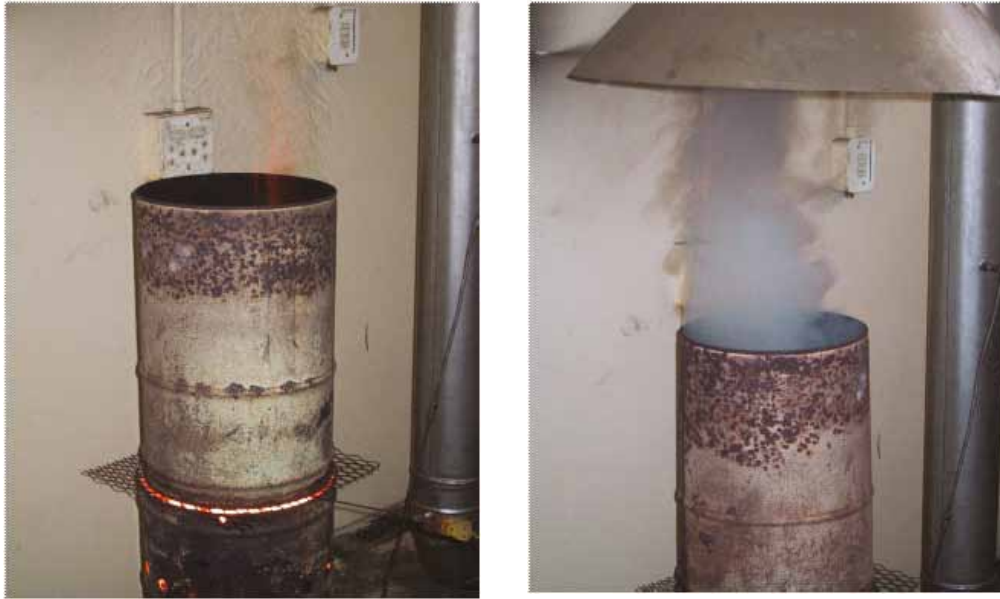
Figure A.5.5. Basa njengo Magogo: Comparative smoke emissions from the Basa njengo Magogo fire (left) and a fire ignited with the bottom-up method (right), using traditional D-grade coal. (Source: CSIR Environmentek (2005).)
