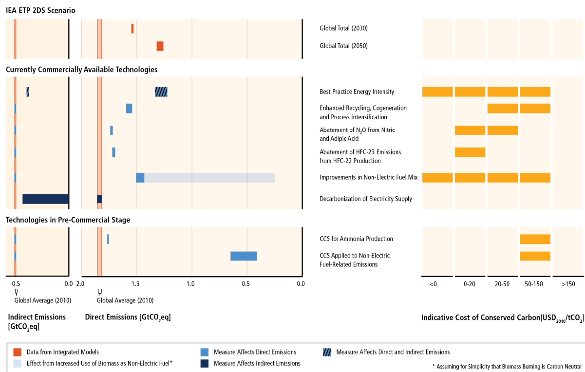
Figure 10.9. Indicative global indirect (left) and direct (right) CO 2 eq emissions and levelized cost of conserved carbon resulting from chemicals production for various production practices/technologies and CO 2 emissions in IEA ETP 2DS scenario (for data and methodology, see Annex III).
